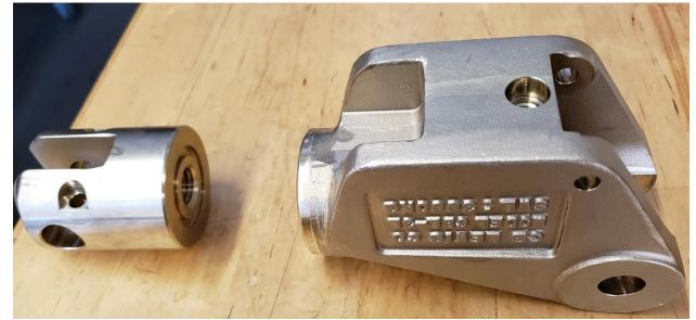
4.12 Use a 1/2" deep well socket to remove the Air Fitting from the body.
