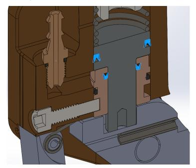
6.6 Assemble the Piston Sub-assembly:
