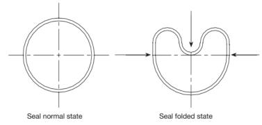
6.5.7 ...then install it in the inside of the Bushing. Be careful not to tear or slice the Rod Seal. IMPORTANT: Make sure the lip of the seal is pointing towards the closer end of the bushing, as shown below (highlighted in blue). This direction may not be intuitive but is best for function.
