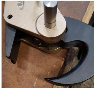
6.11.4 Slide the Hook Pin through the Body and Hook until the Hook Pin is centered in the Body.
