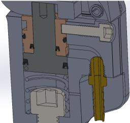
6.5.3 Spray or wipe a light coat of Air Tool Oil into the inside of the Bushing and especially in the seal groove.
