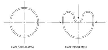
6.5.6 ...then install it in the inside of the Bushing. Be careful to not tear or slice the Rod Seal. IMPORTANT: Make sure the lip of the seal is pointing towards the closer end of the bushing, as shown in 7.5.2 above. This direction is not intuitive but is best for function.
