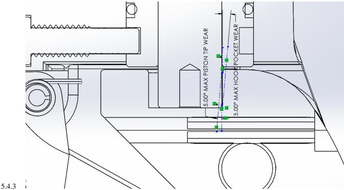
5.5 If the pocket in the 20178 Hook is deformed or worn more than 0.035" or 5 degrees, replace the Hook. The pocket is oval, not round. The pocket can be measured with a caliper to see if the shallow edge of the pocket is more than .035" larger than the deepest portion of the pocket, along the same direction.
